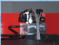
Hydro-Electric Servo Valves Top View-Hoerbiger Hydraulic Module Mounted Directly to Cylinder Heads.
