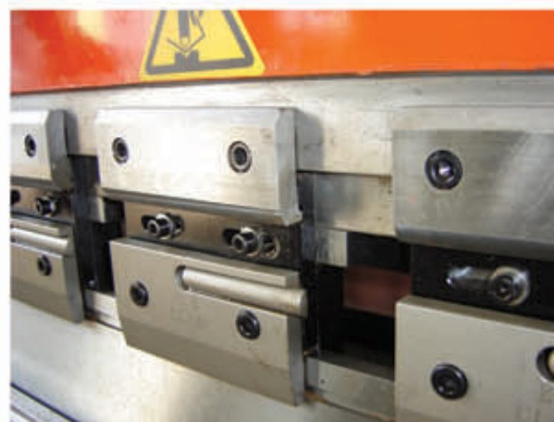
Standard Tool Clamps are precision Euro/ American type with crowning wedges. Other types can be supplied.
