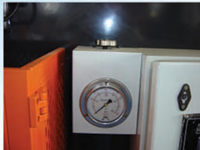
Tonnage can be set to suit the forming operation and protect tooling from overloads.
