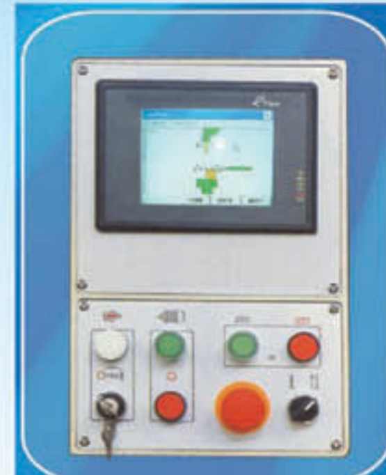
Standard 3 axis CNC control displays Ram depth position on top row and Back Gauge position on the second row. V axis Crowning is included. R axis is optional.
