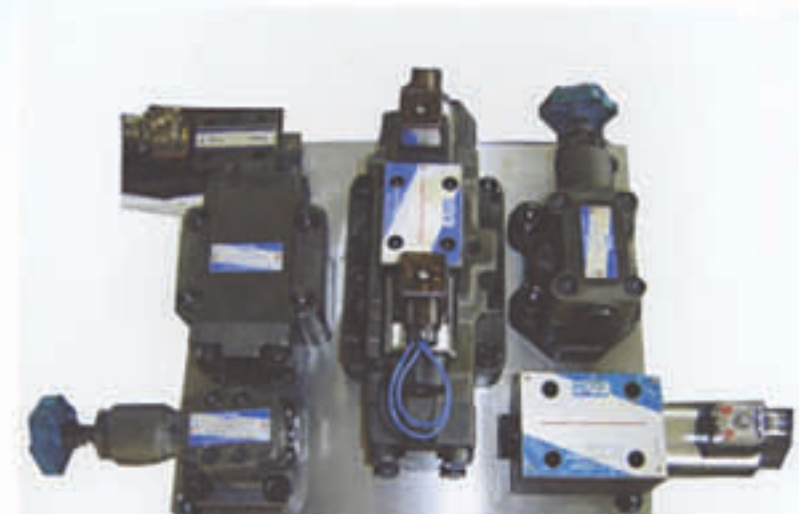
The steel Integrated valve block eliminates most piping and reduces leaks. Service can be accomplished without removing piping.
